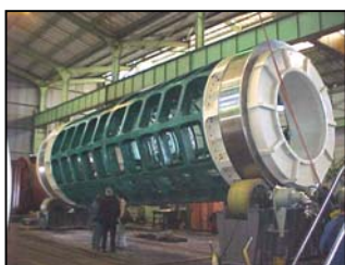
Manufactured trommel on test in factory.
